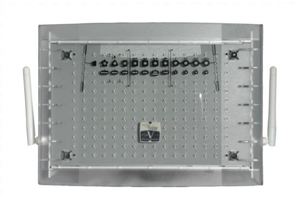
Figure 6: Top view of Teldat-V router with WLAN antennas
