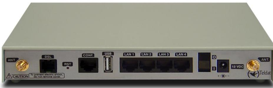
**Figure 5: Teldat C1+L: rear panel.**
