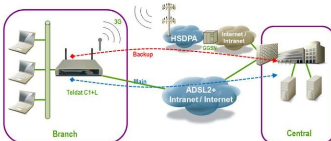
**Figure 2: ADSL2+ connectivity and 3.5G backup**
