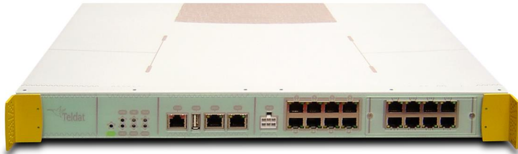
Illustration 6: Atlas-i60/i61 router front panel
